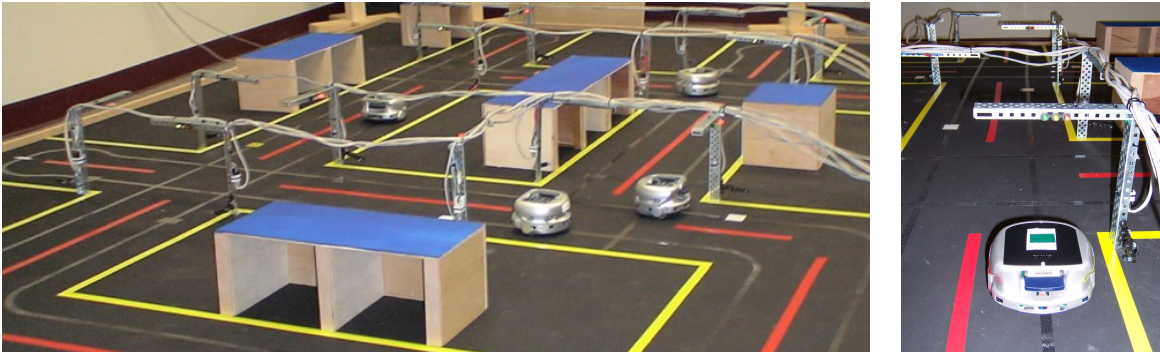
Fig. 1. Robotic Urban-Like Environment (RULE). Left: Khepera III car-like robots move autonomously on streets while staying in their lanes, observing traffic rules, and avoiding collisions. Right: A car waiting at a traffic light.
